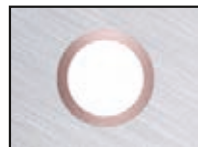
Kupfer-Nickel-Kühlkanal copper-nickel cooling channel
