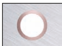
Kupfer-Nickel-Kühlkanal copper-nickel cooling channel
