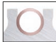
Kupfer-Nickel-Kühlkanal* copper-nickel cooling channel*
