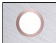
Kupfer-Nickel-Kühlkanal copper-nickel cooling channel
