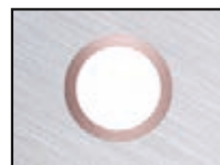
Kupfer-Nickel-Kühlkanal copper-nickel cooling channel
