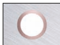
Kupfer-Nickel-Kühlkanal copper-nickel cooling channel
